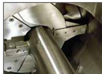
Discharge weir in open position
