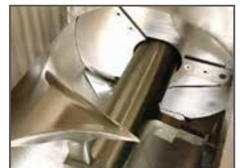
Discharge weir in closed position
