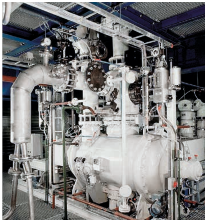
Lödige process unit with heating/cooling jacket for preparing special mixes
