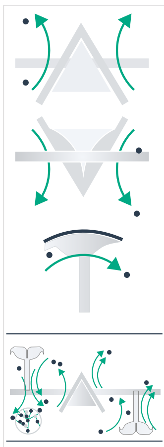
Schematic representation of the fluid bed generated mechanically
