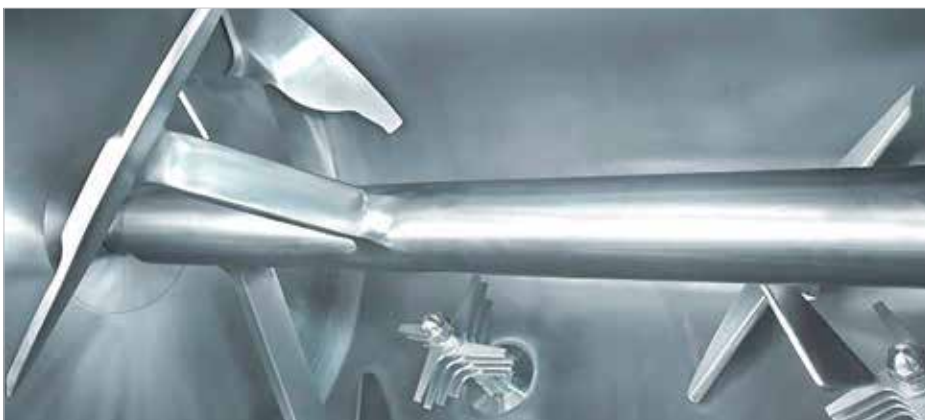
Fully welded mixing elements in hygienic design
