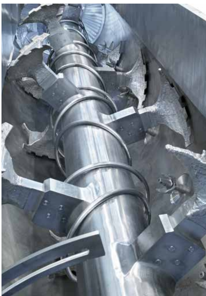
Shaft with cleaning rings
